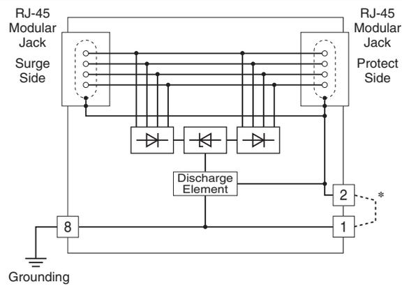
\*Remove the shortcircuit bar when the LAN cable's shield wire is floating.
