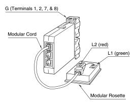
• Shortcircuit Test for the Internal Discharge Element Check resistance across the following terminals on the high resistance range of multimeter (infinite or greater than 100M $\Omega$  standard).
