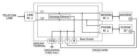
Be sure to cross-wire between G terminals of modem / telephone set and the terminals 2 & 7 of the MD-TL.
