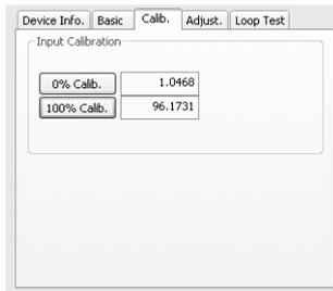
The Potentiometer input can be set from 0% to 100% based on the real input value. When you want to set the present input value to 0%, just push the button “0% Calib.” and the input value in engineering unit is displayed beside the button. Use the same way to set the potentiometer input to 100% by using button “100% Calib.”
