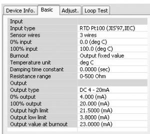
When 'Unlock' box located above Device Info tab is checked, modifiable parameters are highlighted on the light orange background. Click one of such parameters and to show a pull-down list or an edit box to modify it.
