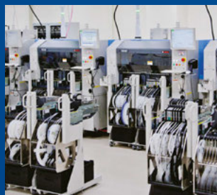
Multiple in-line chip mounters (1st floor)
