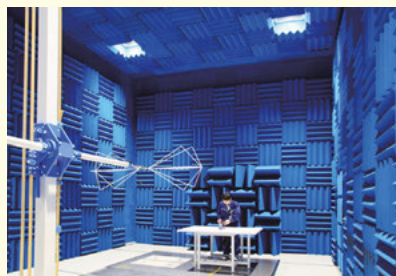
Anechoic chamber certified and registered by the official body (VCCI*2)
