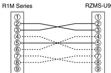
The above connection including solid and broken lines is an example of 'Interlink' cable.
