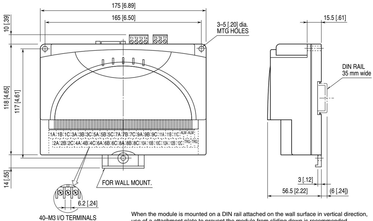
When the module is mounted on a DIN rail attached on the wall surface in vertical direction, use of an attachment plate to prevent the module from sliding down is recommended.
